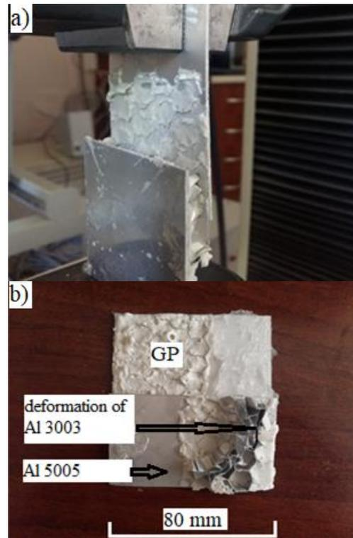
**Figure 4.** Photographs of shear strength measurement; a) during the test, b) deformation on the core aluminum after the test.
