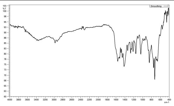
Figure 4. FT-IR spectrum of the L-Ni complex
