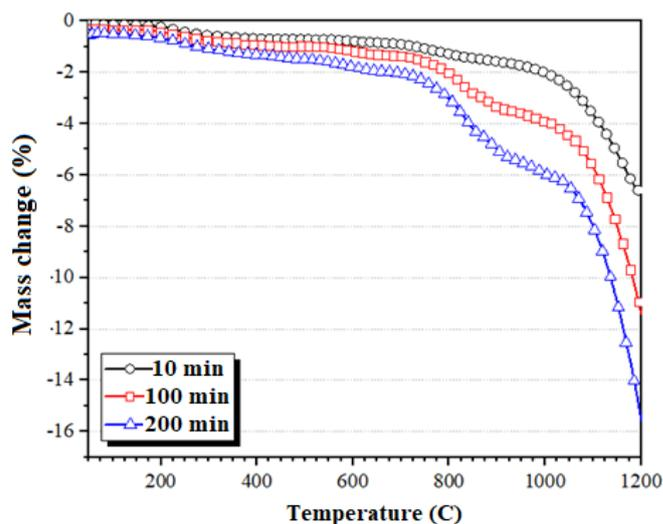
**Figure 7.** TGA curves obtained after the mechanochemical synthesis process at different times.
