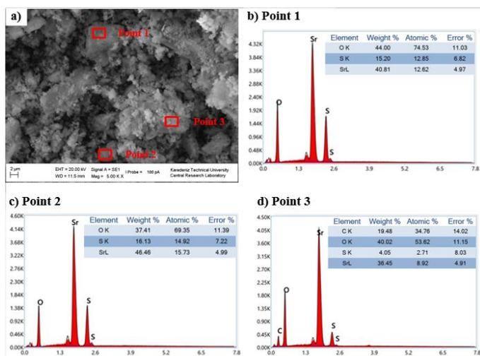
**Figure 3.** EDS results of powders subjected to 10 minute mechanochemical synthesis.
