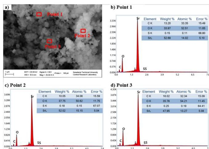
**Figure 4.** EDS results of powders subjected to 200 minute mechanochemical synthesis.
