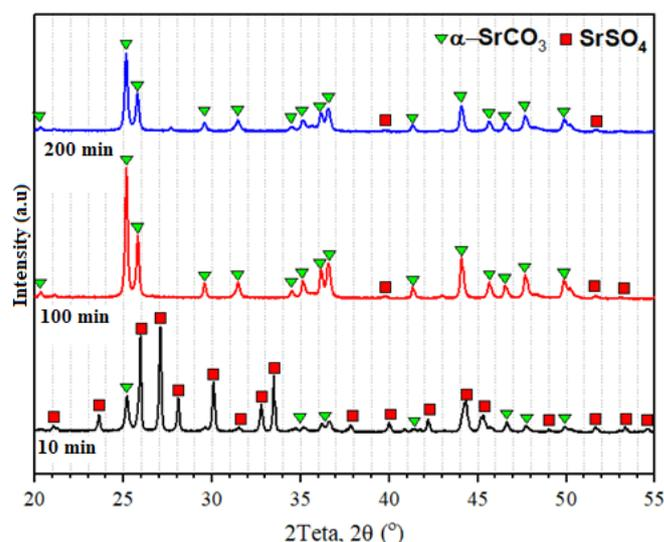
**Figure 5.** The X-ray diffraction patterns obtained after mechanochemical synthesis with different times.
