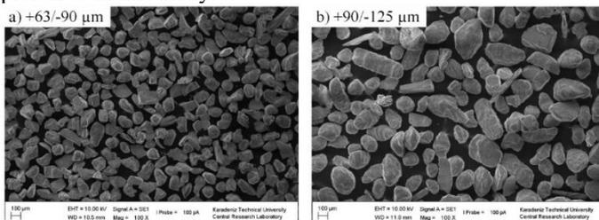
**Figure 1.** Scanning electron microscope (SEM) images of concentrated celestite ore obtained from different sieve intervals.
