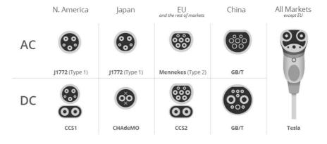
Figure 2. Connector types [22].
