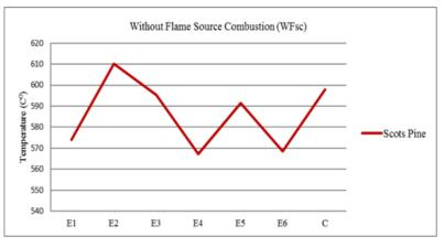
Figure 3. WFsc combustion temperature values of Scots pine test samples according to impregnation compositions
