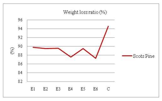
Figure 4. Weight loss ratios of Scots pine test samples according to impregnation compositions
